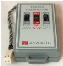
Test temperatures at +50.0°C, 0.0°C and -50.0°C can be simulated on transmitter input 1 to test the alarm. The fob temperature simulator is attached to a connector inside the transmitter unit and a temperature probe bypass switch is thrown. The simulated temperature is selected and will be shown on the display. If this temperature is out with the alarm limits it will activate the relevant alarm after the time delay.
