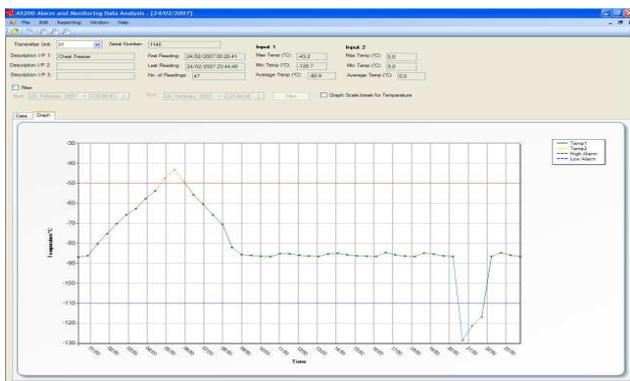
If either I/P1 (Temp1) or I/P2 (Temp2) value goes into the high alarm, the graph line is coloured red. If the input value goes below the low alarm set-point, the graph line is coloured blue.
